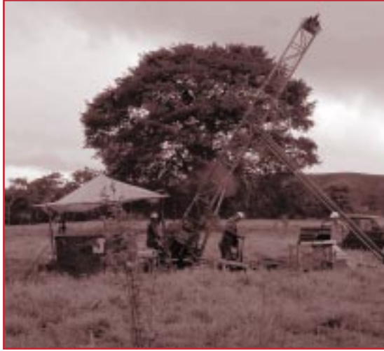
Drilling continues at Sungem to test the eastern soil geochemical anomaly and gossan zone at SG 6.
