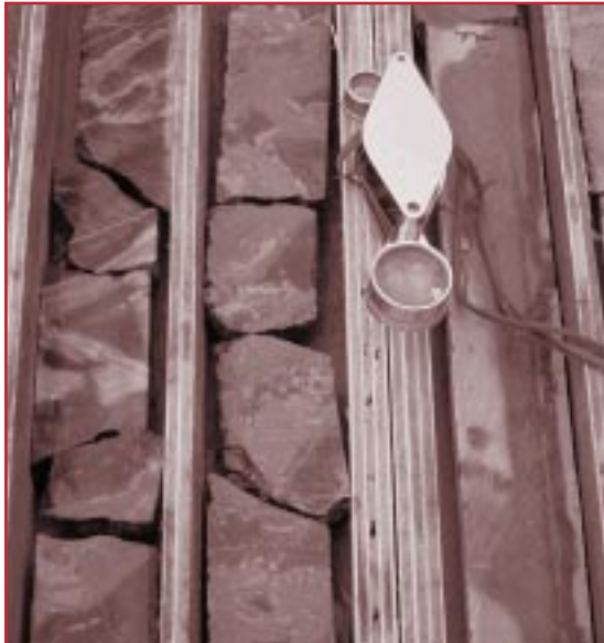
Mineralised core from Sungem Drillhole SG2 at 150m. Massive to semi-massive pyrite and sphalerite, with lesser galena hosted predominantly in dolomite rock and breccia.
